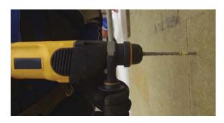
hammer drilling – drilling by rotation with a small number of high energy strikes with the drill bit into the substrate; recommended for drilling in extremely hard structures such as concrete;
