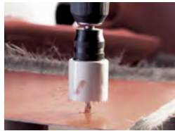
HSS bi-metal with 8% cobalt. Progressive tooth strip.
