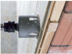
Diamond-ground tungsten carbide teeth, drop-shaped chip clearance slots.
